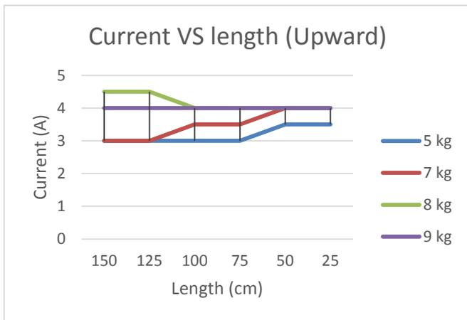
FIGURE 14: Current used by the motor to move the fan upward with different load
