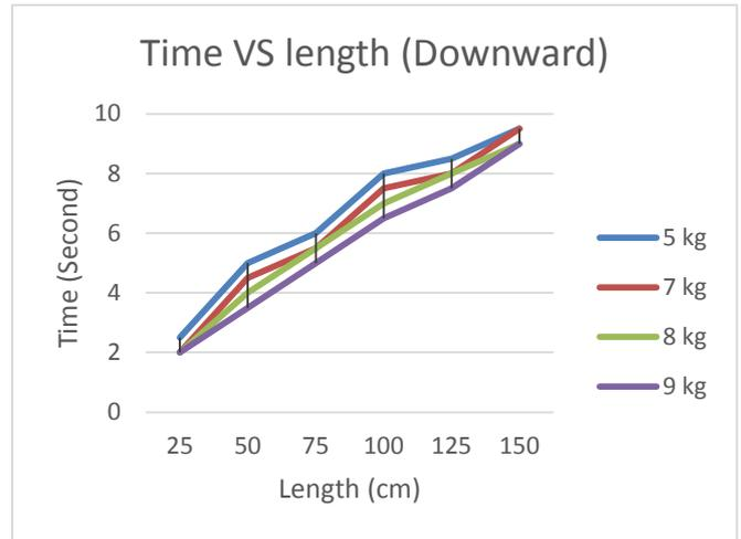
FIGURE 11. Time taken to move the fan downward with different load
