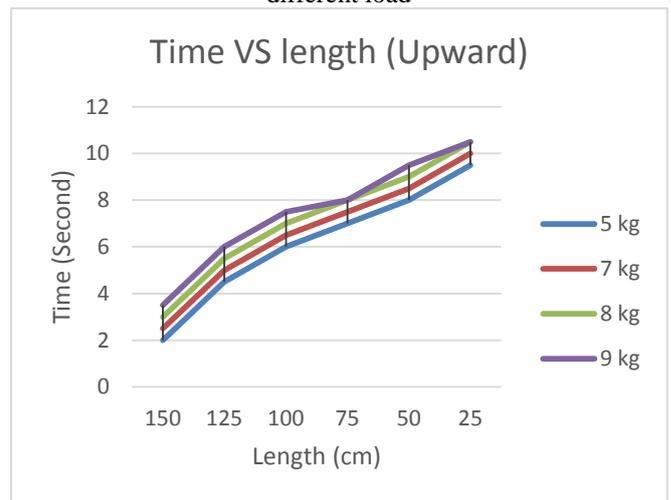
FIGURE 12. Time taken to move the fan upward with different load
