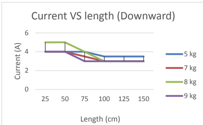
FIGURE 13: Current used by the motor to move the fan downward with different load
