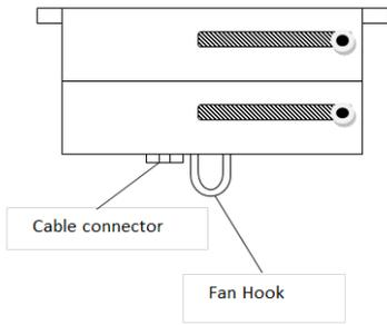
FIGURE 2. Conceptual design (Side View – Close Position)
