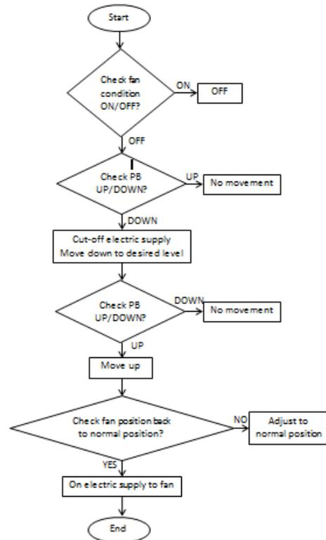
FIGURE 5. System Design Flowchart
