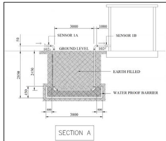
Figure 2: Experiment layout with waterproof barrier
