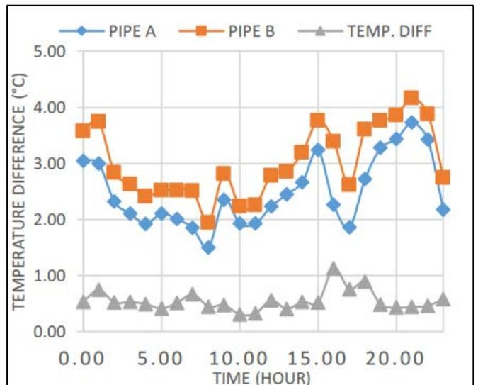
Figure 7: Temperature difference for both pipe setups at 11th November 2015
