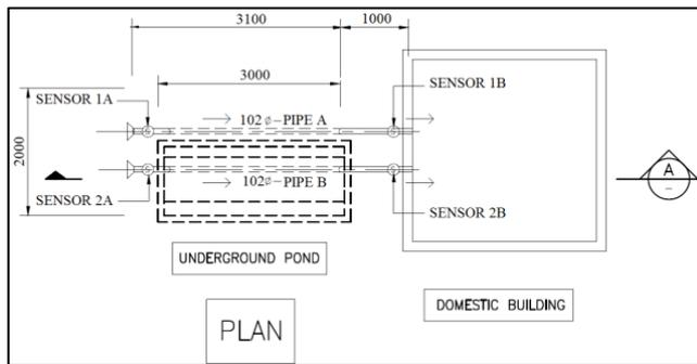
Figure 1: Apparatus setup layout plan (Top View)
